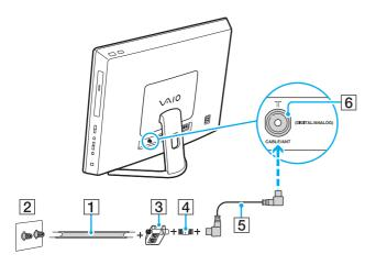
To connect to an antenna (air) for digital television system (ATSC signal standard)
